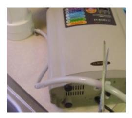
Cut hose from prefilter (or from saddle valve if no prefilter) at the desired length. Leave some slack for final positioning. This end will attach onto lon Farm water input.
