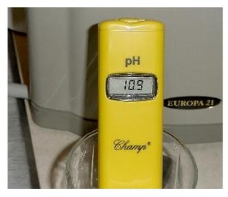
Use included pH test drops, or pH meter to measure pH prior to consumption. Read Ion Farm manual, section 2 for more information about pH adjustment.
