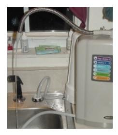
Upon power-up, the lon Farm will play a tune while it automatically cleans. When music stops, alkaline water is dispensed from the flex hose. Push power button to turn off water. (Note, water-flow may take several seconds at first usage. You may also notice water discoloration as carbon fines wash out of new filter.
