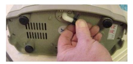
Remove dust caps from Ion Farm water input and acid water output.
