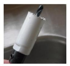
You will need a 1 inch hole saw, suitable for stainless steel sink. Depending on the installation, you may decide to drill through counter instead.
